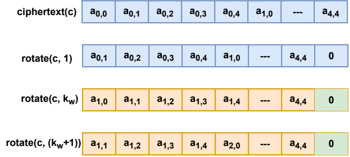
Fig. 3: Rotated Ciphertexts for convolution. The number of rotations is a total of k^2 - 1 where k is the kernel width.
