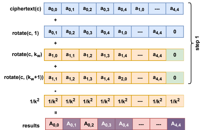
Fig. 5: Vector Encoding Secure Average Pooling: These rotations are then summed and multiplied by 1/k^2
