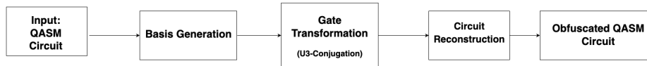
Fig. 1. Workflow of the proposed quantum circuit obfuscation using U3 -conjugation. The process begins with a QASM circuit, applies a randomized basis transformation, transforms each gate, and restores the original basis to produce an obfuscated circuit with preserved functionality.
